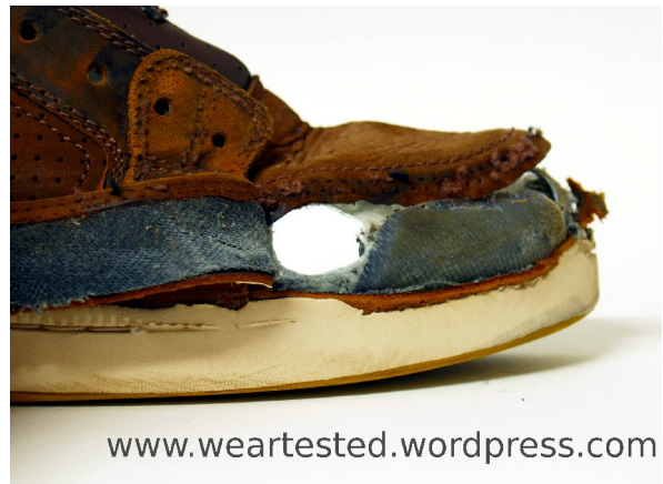
Hole in the inner material, too short plastic reinforcement
